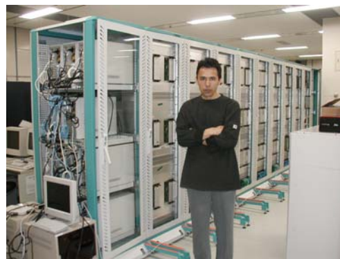
Fig. 18. Molecular Dynamics Machine (78 TFLOPS) [33] with Dr. Kholmurodov at Computational Science Division, RIKEN.
